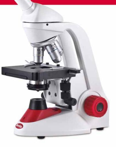
**The integrated mechanical stage** allows the sample to be moved accurately in the X and Y direction. The possibility of moving the sample around with great precision will be even more appreciated when using the included 100X-Oil objective. This means that a total magnification of 1000X can be reached.
