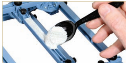
Step 2: Insert rebar into tensioning apparatus and pour a mixture of sand and plaster of Paris into the mold.
